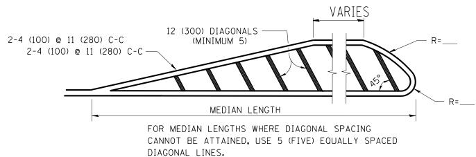
DIAGONAL LINE SPACING: 50' (15 m) C-C (LESS THAN 30MPH (50 km/h)) 75' (25 m) C-C 30MPH (50 km/h) TO 45MPH (70 km/h)) 150' (45 m) C-C (MORE THAN 45MPH (70 km/h))
