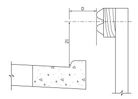
Note: If it is necessary for D to be more than 12 and less than 10'-0" type M-2 curb and gutter (Std. 606001) shall be used in front of and in advance of the guardrail.
