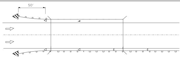
Reflectors are not to be placed on Terminal End Sections. (min. 3 reflectors regardless of length).
