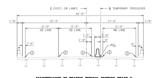
MAINTENANCE OF TRAFFIC TYPICAL SECTION-STAGE II **EXISTING SOUTHBOUND IL 116 STRUCTURE OVER TEN MILE CREEK** (LOOKING NORTH)
