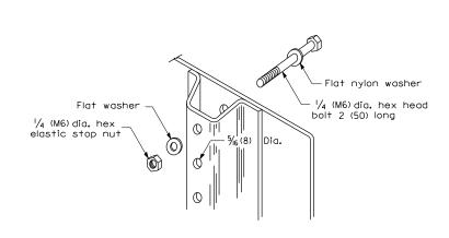
DETAIL OF MOUNTING TERMINAL MARKER TO POST
