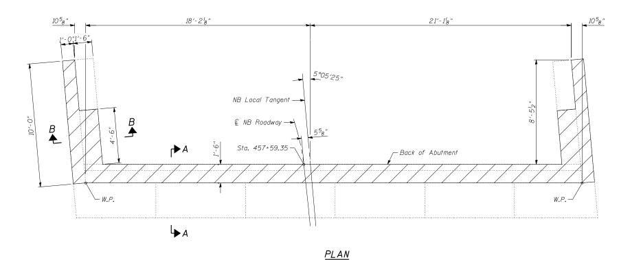
\* Existing reinforcement bars in abutment backwall shall be cut to fit proposed construction.
