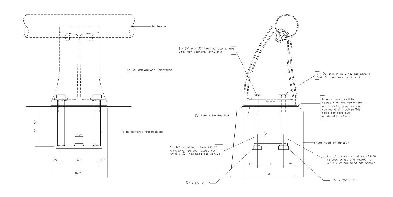
Note: New Rail Post anchorage devices will be required at each location where posts are connected to new construction. Cost shall be included with Concrete Superstructure.
