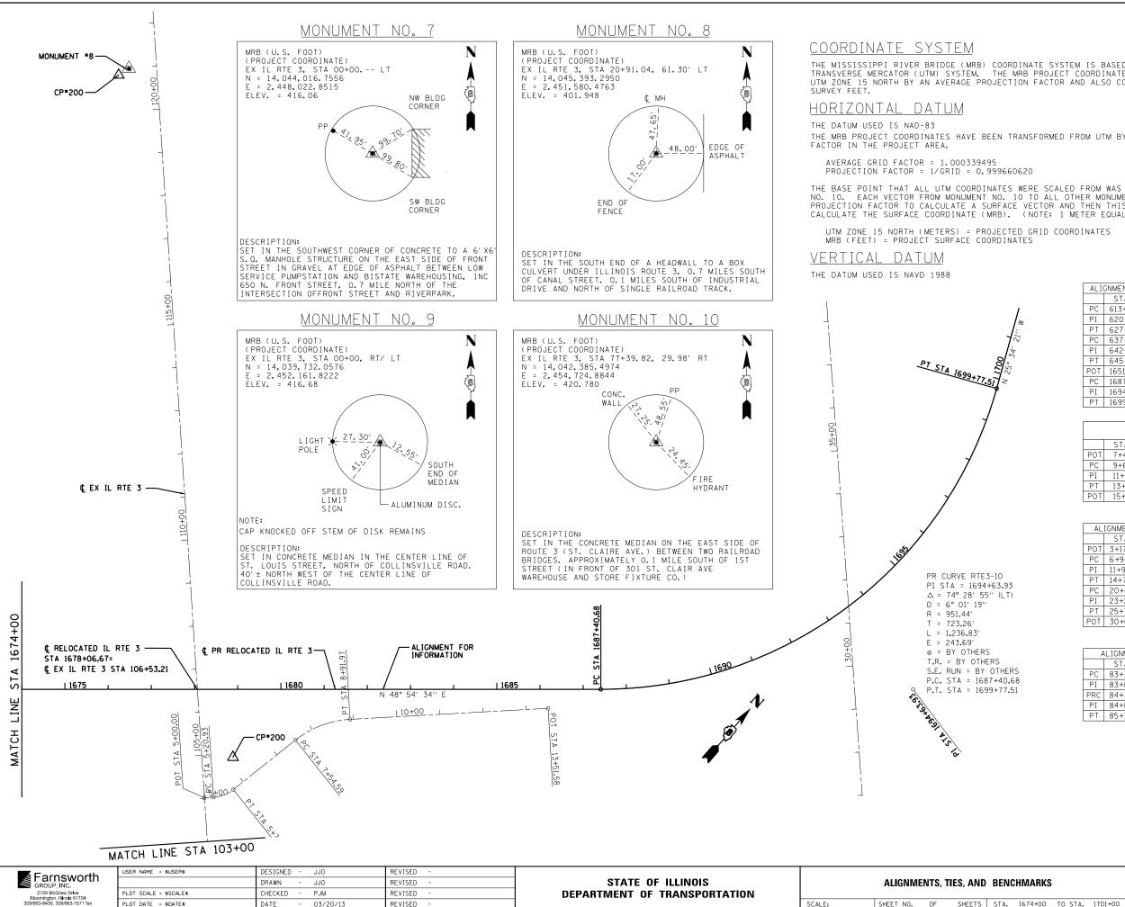
THE MISSISSIPPI RIVER BRIDGE (MRB) COORDINATE SYSTEM IS BASED ON A MODIFIED UNIVERSAL TRANSVERSE MERCATOR (UTM) SYSTEM. THE MRB PROJECT COORDINATE SYSTEM HAS CONVERTED FROM UTM ZONE 15 NORTH BY AN AVERAGE PROJECTION FACTOR AND ALSO CONVERTED FROM METERS TO U.S.
