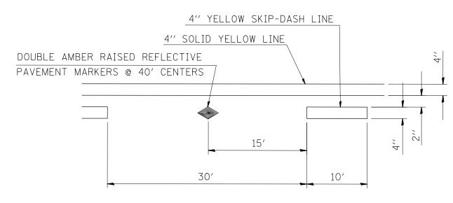
TYPICAL APPLICATION FOR SOLID YELLOW AND SKIP-DASH LINES WITH RAISED REFLECTIVE PAVEMENT MARKERS
