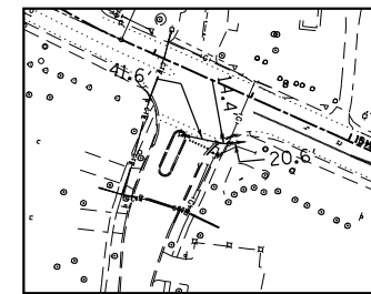
CONTROL POINT 3 CUT "X" IN SIDEWALK STA. 13+94.58, 49.93' RT ELEV. 742.54
