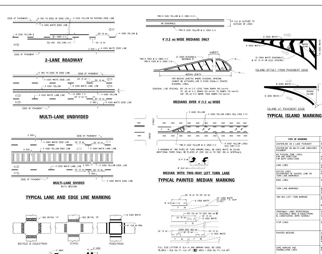
\* TURN LANES IN EXCESS OF 400' (120 m) IN LENGTH MAY HAVE AN ADDITIONAL SET OF ARROW - "ONLY" INSTALLED MIDWAY BETWEEN THE OTHER TWO SETS OF TYPICAL LEFT (OR RIGHT) TURN LANE TYPICAL TURN LANE MARKING
