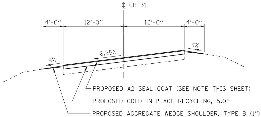
**PROPOSED TYPICAL SUPERELEVATION SECTION**
