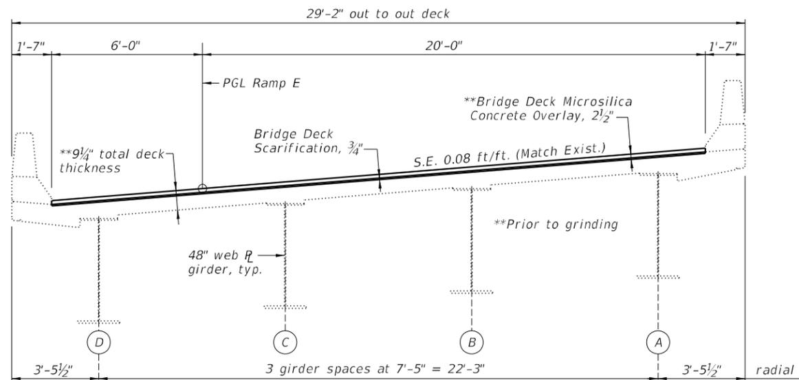
**CROSS SECTION THRU BRIDGE DECK**
