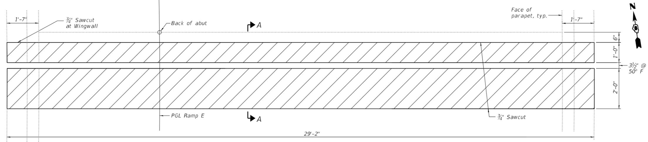
**ABUTMENT NO. 1 PLAN SHOWING JOINT REMOVAL**
