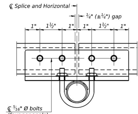
Sign shall be even with the top of the bracket, but it may extend no more than 6" above the top of the bracket for field adjustments.
