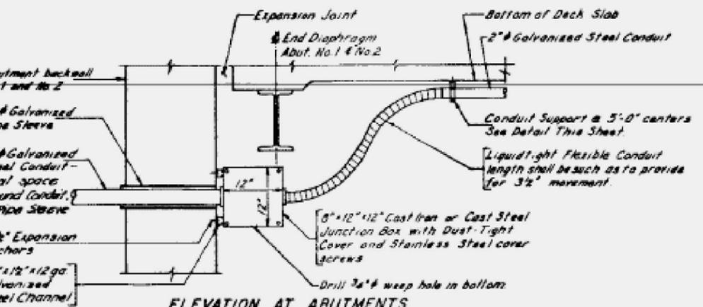
**ELEVATION AT ABUTMENTS**
