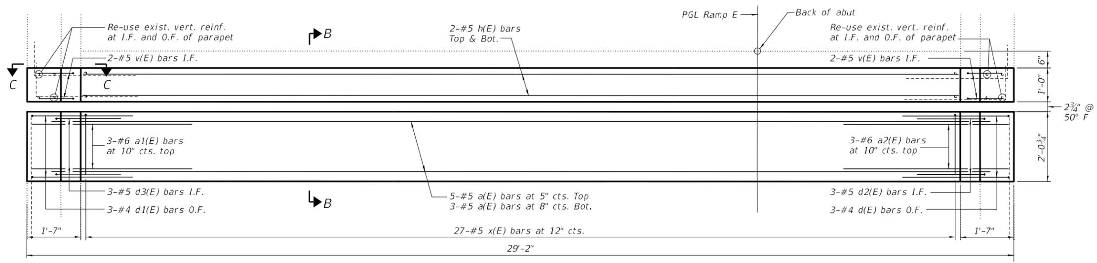
**ABUTMENT NO. 2 PLAN SHOWING JOINT REPLACEMENT**
