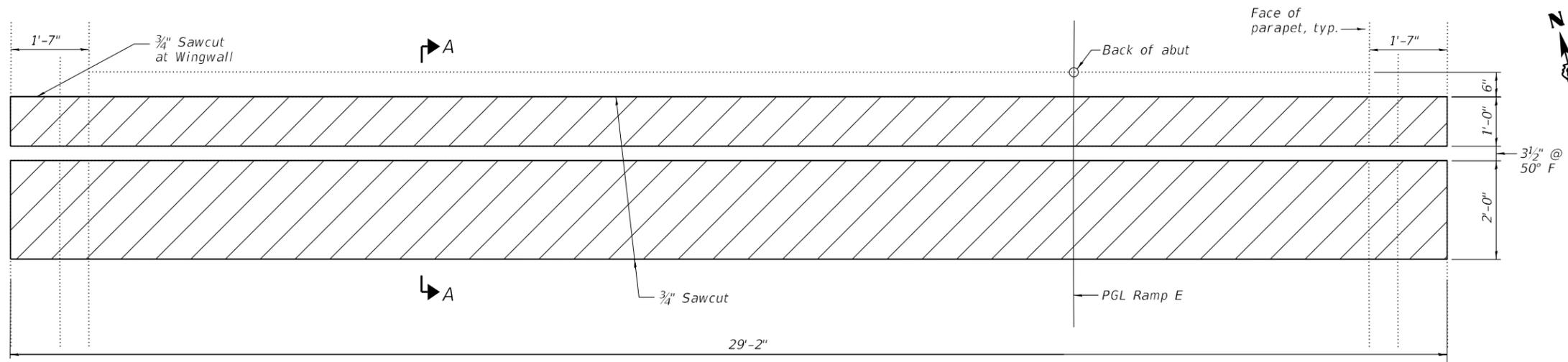
**ABUTMENT NO. 2 PLAN SHOWING JOINT REMOVAL**
