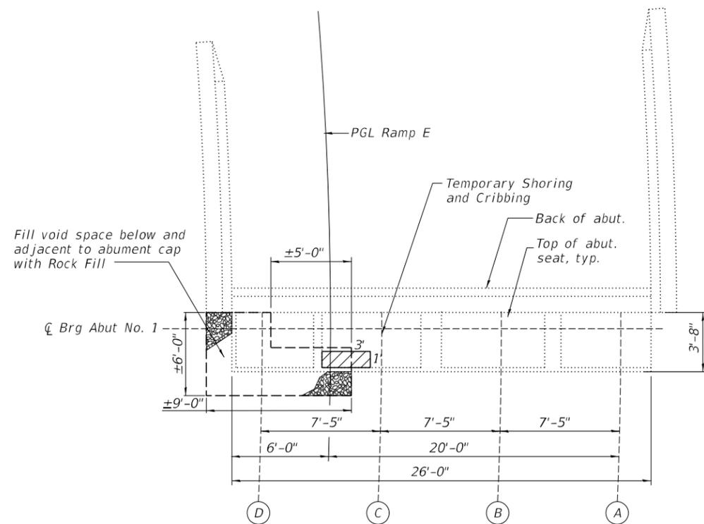
**ABUTMENT NO. 1 REPAIRS - PLAN**
