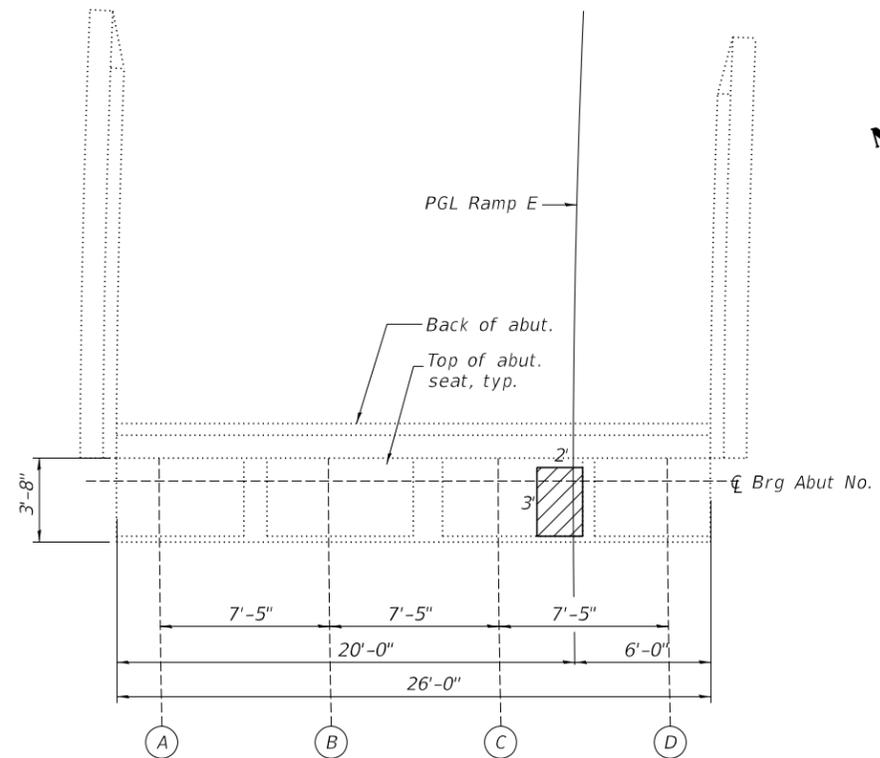
**ABUTMENT NO. 2 REPAIRS - PLAN**
