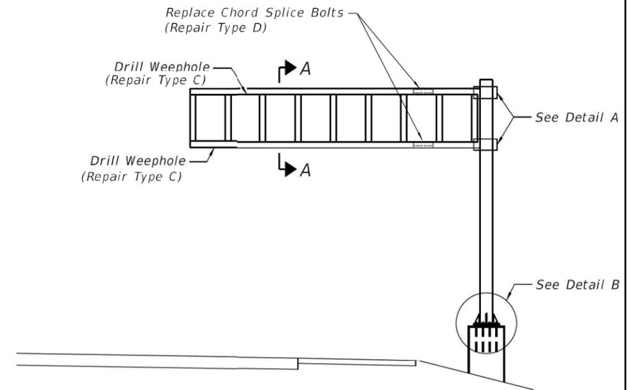
**CANTILEVER SIGN STRUCTURE - ELEVATION**
