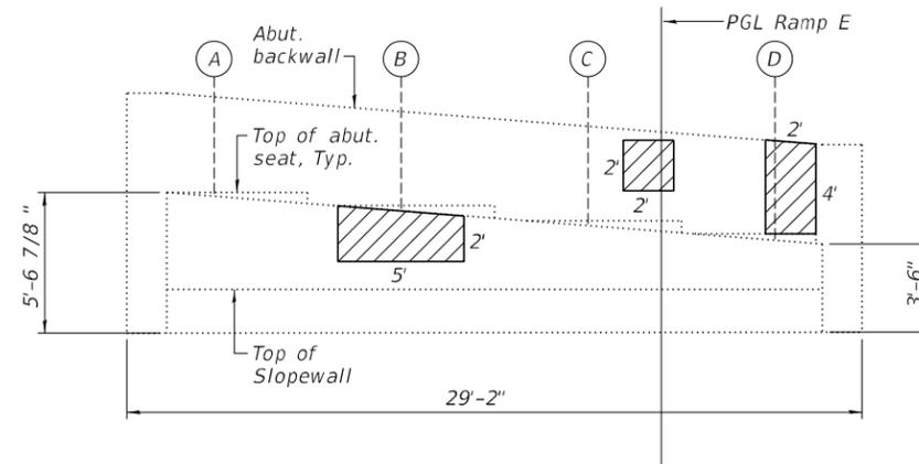
**ABUTMENT NO. 2 REPAIRS - ELEVATION**
