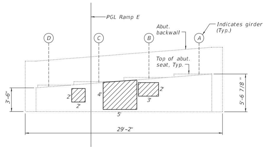
**ABUTMENT NO. 1 REPAIRS - ELEVATION**
