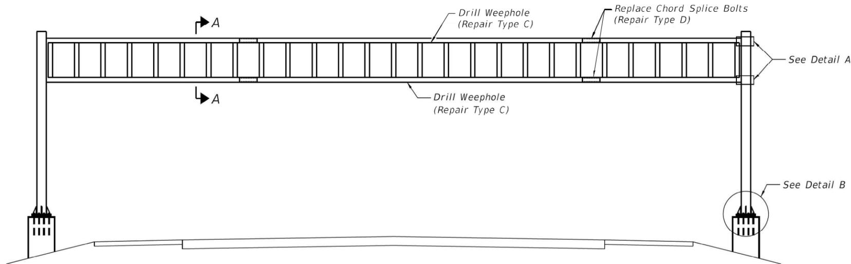
**SPAN SIGN STRUCTURE - ELEVATION**
