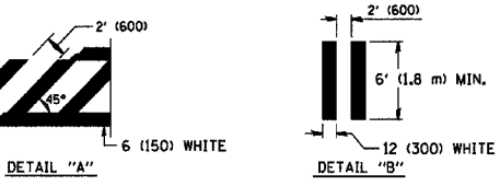
TYPICAL CROSSWALK MARKING
