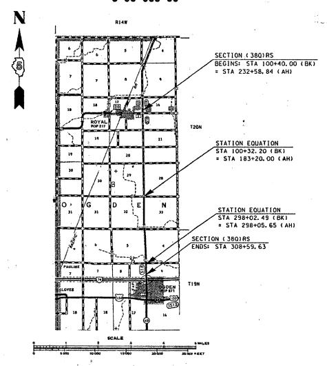
TOTAL LENGTH OF SECTION & PROJECT = 25763.11 FEET = 4.879 MILES NET LENGTH OF SECTION & PROJECT = 25763.11 FEET = 4.879 MILES
