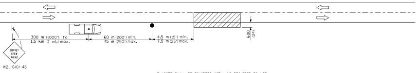
FLAGGER SHALL BE EQUIPPED WITH AND REQUIRED TO USE A HIGH INTENSITY, OR HIGH PERFORMANCE "STOP - SLOW" TRAFFIC CONTROL PADDLE. FLAGGER AND LIGHTING INSPECTOR SHALL BE REQUIRED TO WEAR A HIGH VISIBILITY, REFLECTIVE ORANGE VEST AND EITHER A HARD HAT OR AN ORANGE CAP.
