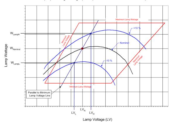
$$Ballast \ Regulation = \frac{\textit{W}_{\textit{LampH}} - \textit{W}_{\textit{LampL}}}{\textit{W}_{\textit{LampN}}} \times 100 \quad \text{, where:}$$
