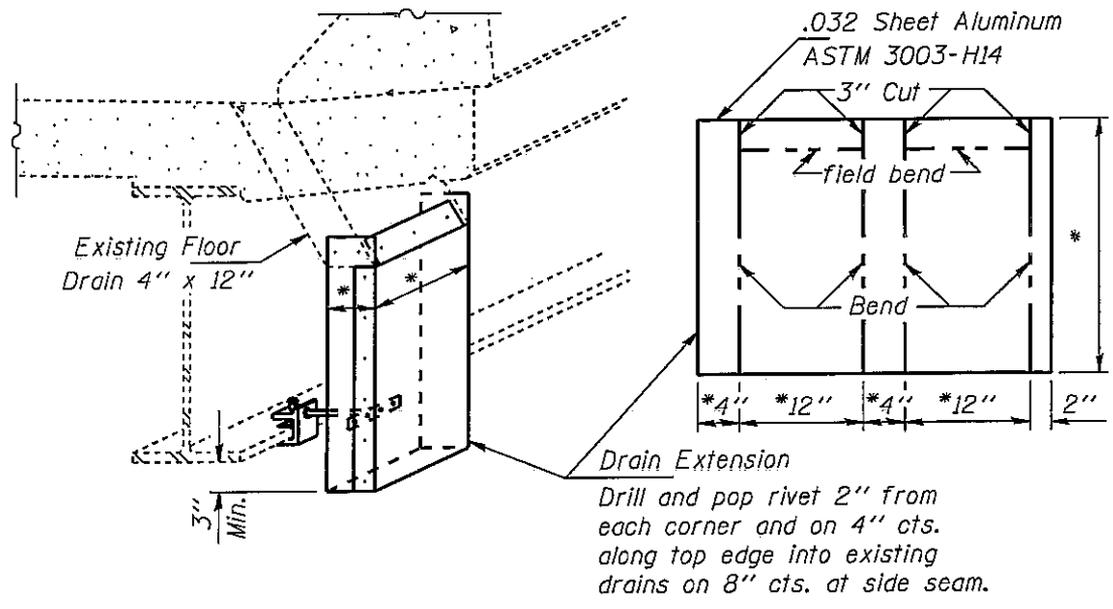
Drill and pop rivet 2" from each corner and on 4" cts. along top edge into existing drains on 8" cts. at side seam.
