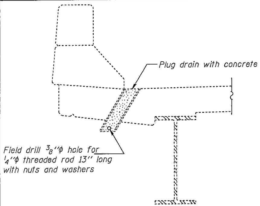
Field drill  $\frac{3}{8}$ "  $\phi$  hole for  $\frac{1}{4}$ "  $\phi$  threaded rod 13" long with nuts and washers
