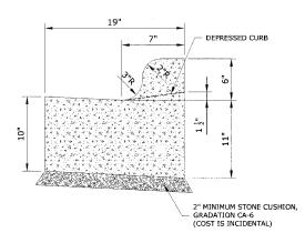
**COMBINATION CONCRETE CURB & GUTTER** TYPE B-6.12 (MODIFIED)
