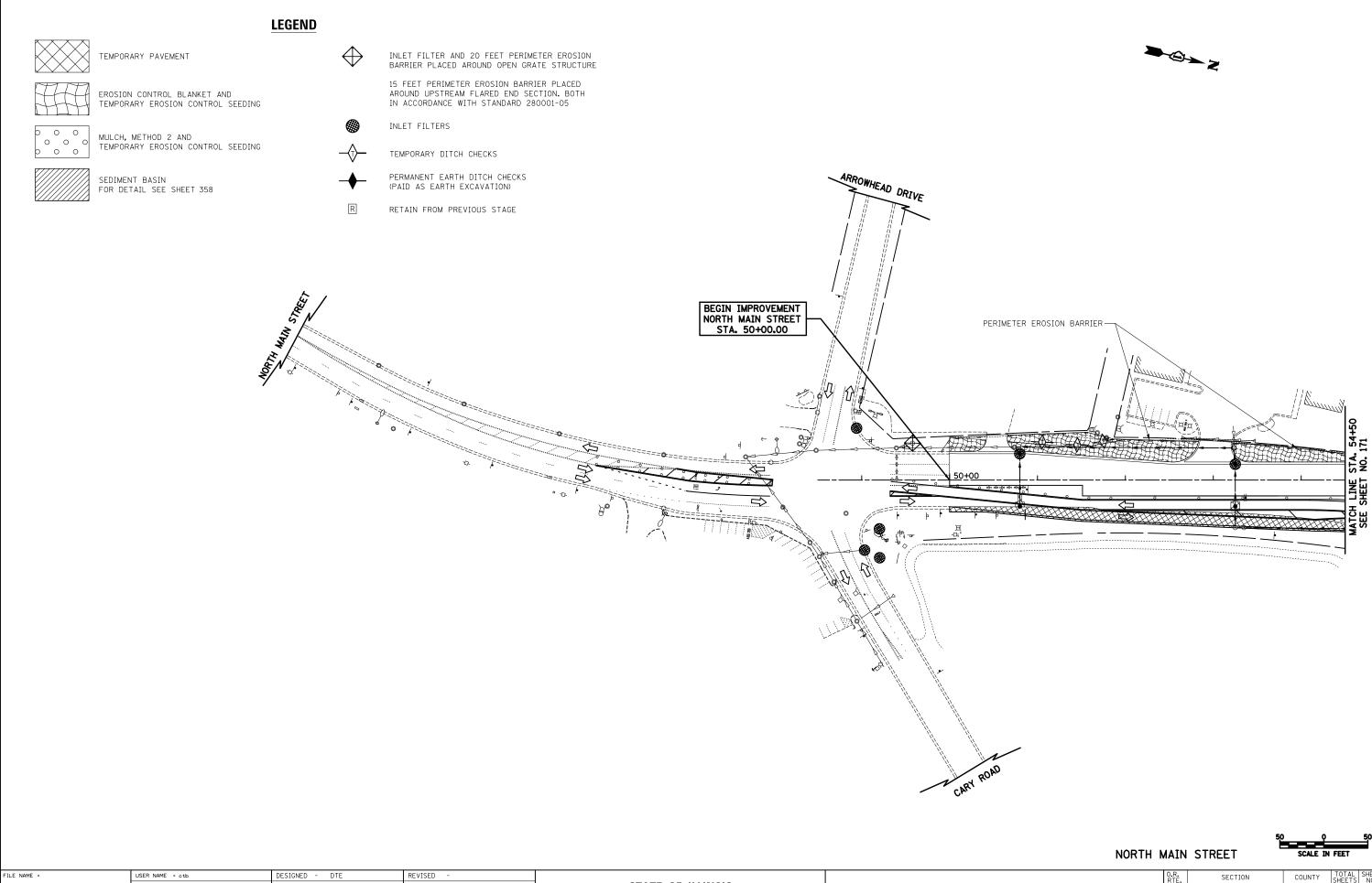
STATE OF ILLINOIS **EROSION AND SEDIMENT CONTROL - STAGE 4A** ...\D160F72-sht-eros-22.dgn DRAWN - DTE REVISED MCHENRY 825 170 0003 18A-2 CHECKED -GAB REVISED **DEPARTMENT OF TRANSPORTATION** CONTRACT NO. 60F72 PLOT DATE = 5/2/2012 DATE 5/3/2012 REVISED SCALE: 1" = 50' SHEET NO. 22 OF 28 SHEETS STA. 50+00 TO STA. 54+50
