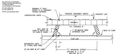
CONSTRUCTION JOINTS SHALL BE PLACED IN A UNIFORM MANNER THAT ALLOWS NO SINGLE SLAB BE MORE THAN 10 FOOT BY 10 FOOT DIMENSIONALLY
