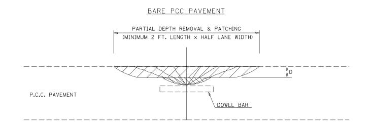
ALL VOLUME OF PARTIAL DEPTH REMOVAL SHALL BE REPLACED WITH HOT-MIX ASPHALT (HMA) AND PAID FOR AT THE CONTRACT UNIT PRICE PER TON FOR PARTIAL DEPTH PATCHING.
