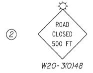
Post mounted sign with Type A Flashing Light
