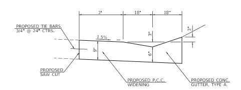
NOTE: THE PROPOSED P.C.C WIDENING AND PROPOSED CONCRETE GUTTER, TYPE A SHALL BE POURED MONOLITHICALLY AND PAID FOR AS CONCRETE GUTTER, TYPE A (SPECIAL).
