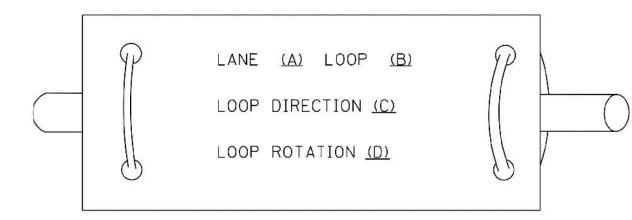
A. LANE 1 IS THE LANE CLOSEST TO THE CENTERLINE OF THE ROADWAY B. LOOP #1 IS THE LOOP IN THE LANE CLOSEST TO THE INTERSECTION. C. LABEL LOOP CABLE "IN" OR LOOP CABLE "OUT".
