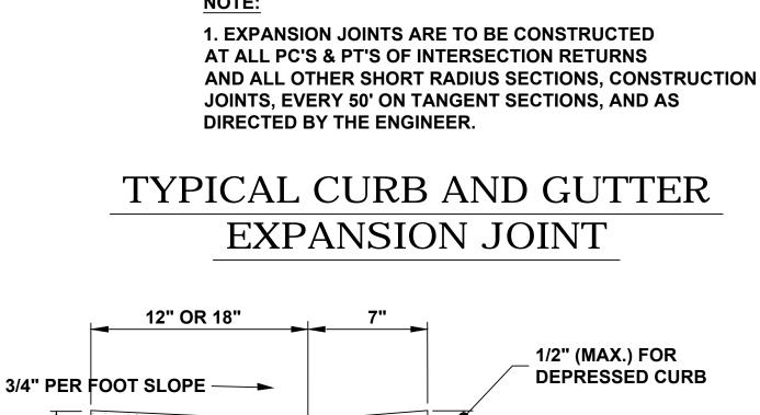
**CROSS SECTION. TRIM ANY EXCESS** 3/4" DIAMETER x 18" EPOXY
