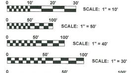
FULL SIZE PLANS HAVE BEEN PREPARED USING STANDARD ENGINEERING SCALES. REDUCED SIZED PLANS WILL NOT CONFORM TO STANDARD SCALES. IN MAKING MEASUREMENTS ON REDUCED PLANS, THE ABOVE SCALES MAY BE USED.
