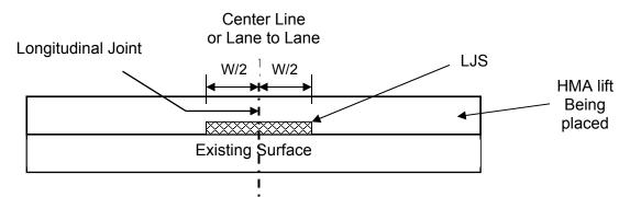
The LJS application shall be centered under the joint of the HMA lift being constructed within 2 in. (50 mm) of the joint.
