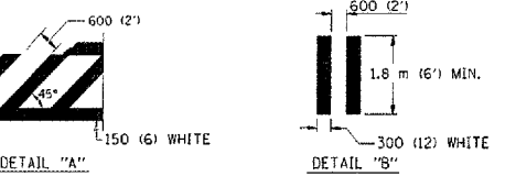
TYPICAL CROSSWALK MARKING
