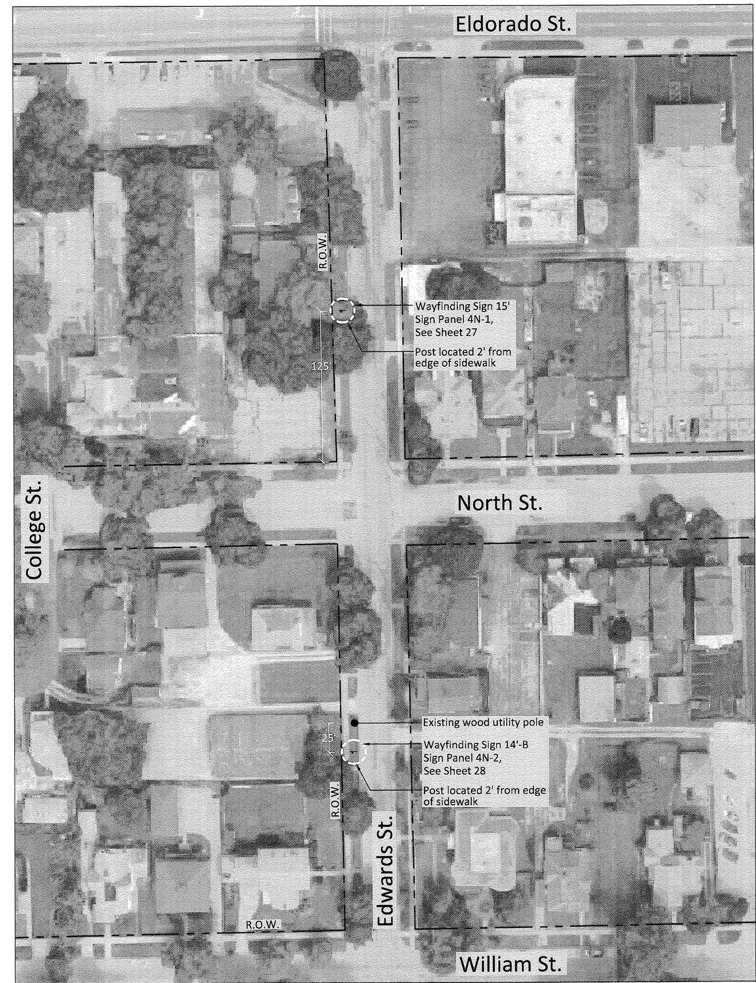
Wayfinding Signs 4N-1 and 4N-2
