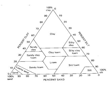
The mechanical analysis should show that the % sand, % silt, and the % clay must yield a silt loam soil. See the attached Textural Classes diagram above. To determine the class plot a line parallel to the % clay axis starting the line at the value of the % silt. Plot another line parallel to the % sand axis starting the line at the value of the % clay. The intersection of these lines should be in the silt loam or loam region, for the soil to be approved.
