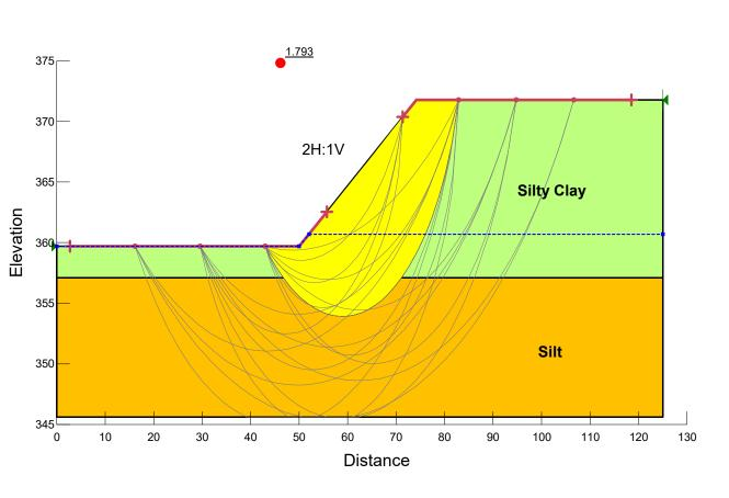
Name: Silty Clay Model: Mohr-Coulomb Unit Weight: 120 pcf Cohesion': 100 psf
