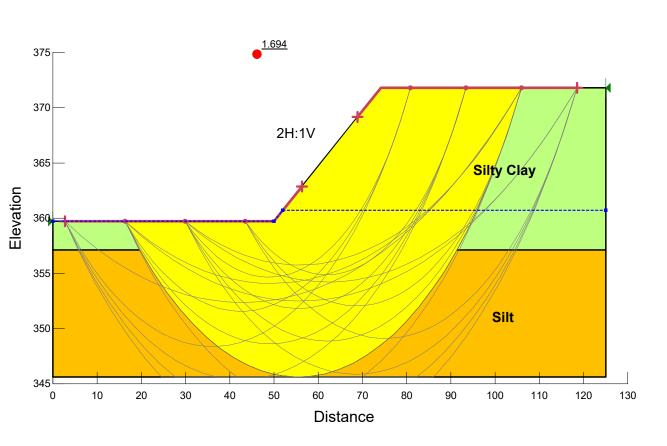
Name: Silty Clay Model: Mohr-Coulomb Unit Weight: 120 pcf Cohesion': 1,080 psf
