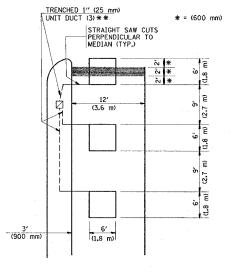
\*\* UNIT DUCT IS TO BE SHOWN ON PLAN SHEETS BUT SHALL NOT BE INCLUDED IN THE PAY ITEMS. NOTE: DUAL LEFT TURNS NOT SHOWN REFER TO PLAN SHEET FOR DETECTOR LOOP REPLACEMENT LEFT TURN LANES WITHOUT MEDIANS
