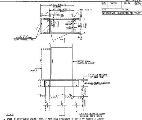
BASED ON CONTROLLER CABINET TYPE IV WITH BASE DIMENSIONS OF 26" x 44" (660mm x 1118mm).
