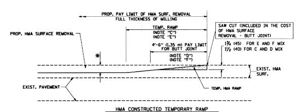
(FOR BUTT JOINT AND HMA TAPER SEE DETAIL BELOW)
