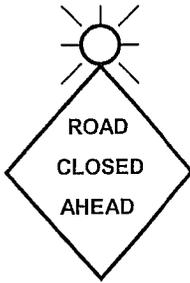
Post mounted sign with Type A Flashing Light
