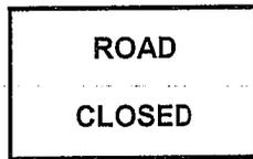
Use with Type III Barricades as shown on Std. 701901 Detail for "ROAD CLOSED TO ALL THRU TRAFFIC". Each Type III Barricade shall have one Type A Flashing Lights, and a minimum of four (4) sandbags.
