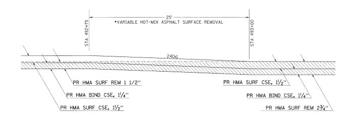
\* VARIABLE DEPTH HOT-MIX ASPHALT SURFACE REMOVAL WILL BE PAID FOR AS HOT-MIX ASPHALT SURFACE REMOVAL 1 1/2"
