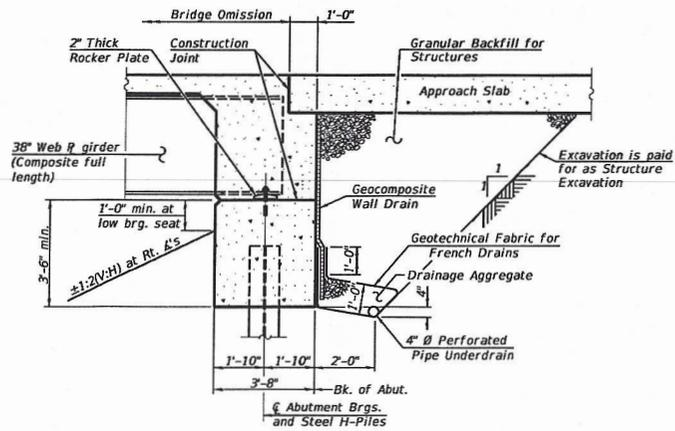
**SECTION THRU INTEGRAL ABUTMENT**
