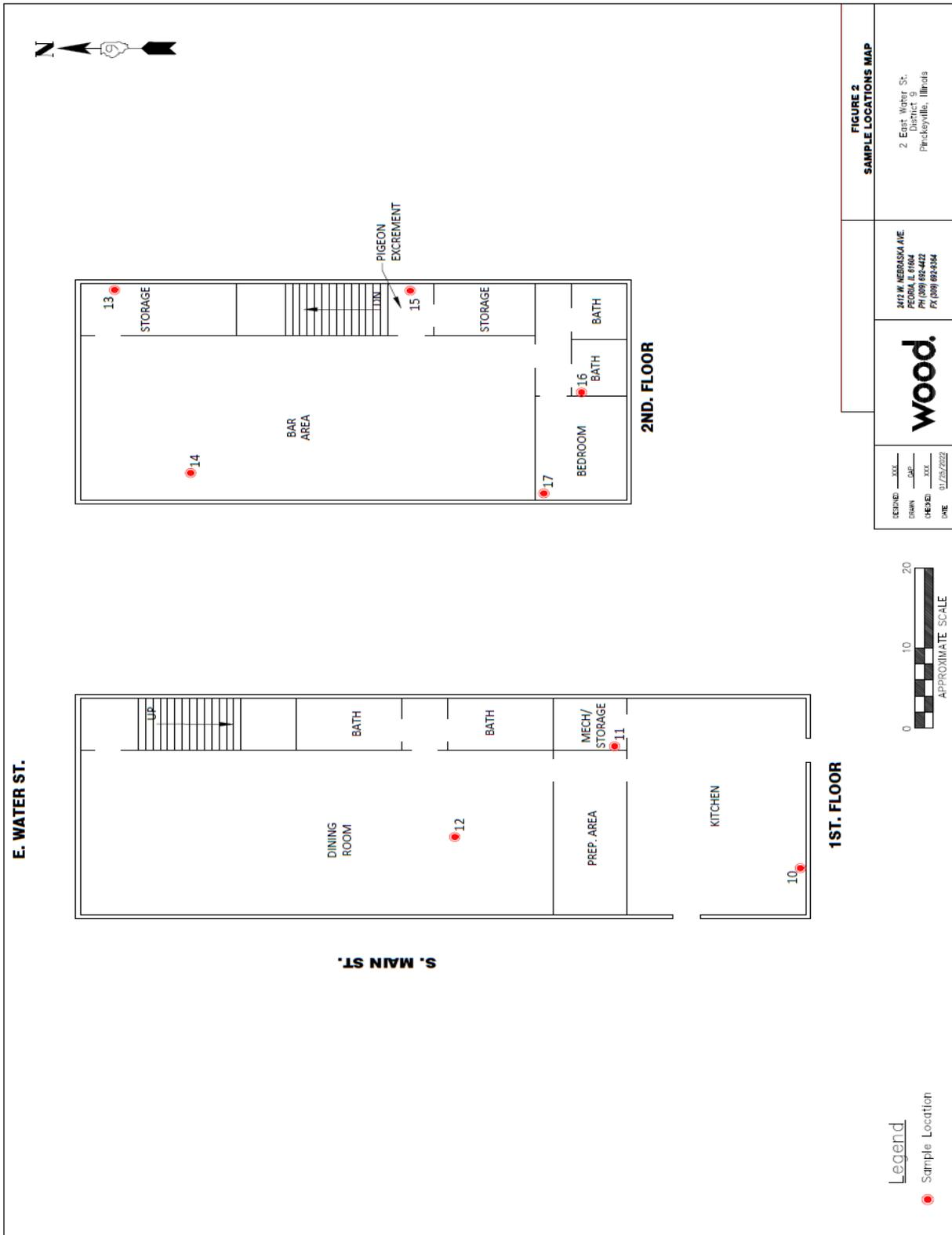
Figure 2- 2 East Water Street, Note: ACM Material Located at Sample Location 14
