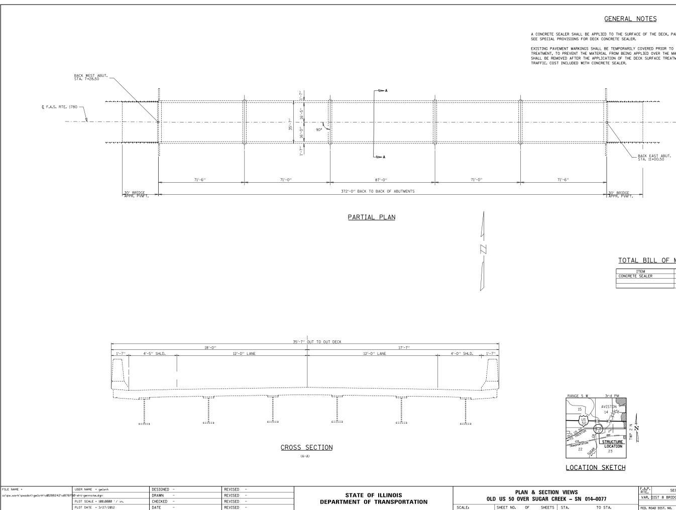
A CONCRETE SEALER SHALL BE APPLIED TO THE SURFACE OF THE DECK, PARAPETS, AND APPROACH PAVEMENTS. SEE SPECIAL PROVISIONS FOR DECK CONCRETE SEALER.
