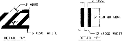
TYPICAL CROSSWALK MARKING
