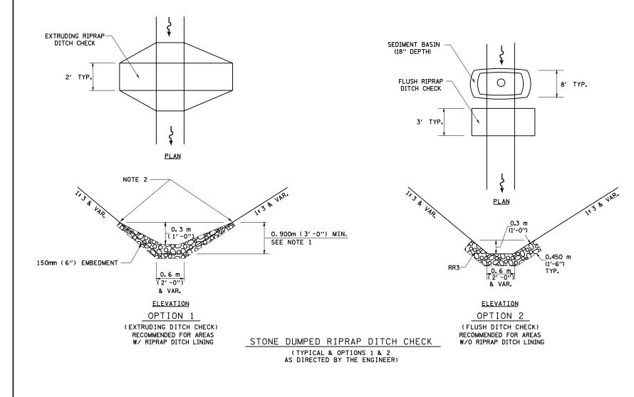
NOTE 1: RIPRAP SHALL EXTEND FAR ENOUGH UP THE SLOPES TO ALLOW O.3m (1') OVERTOPPING TO AVOID ERODING AROUND THE EDGES OF THE RIPRAP.
