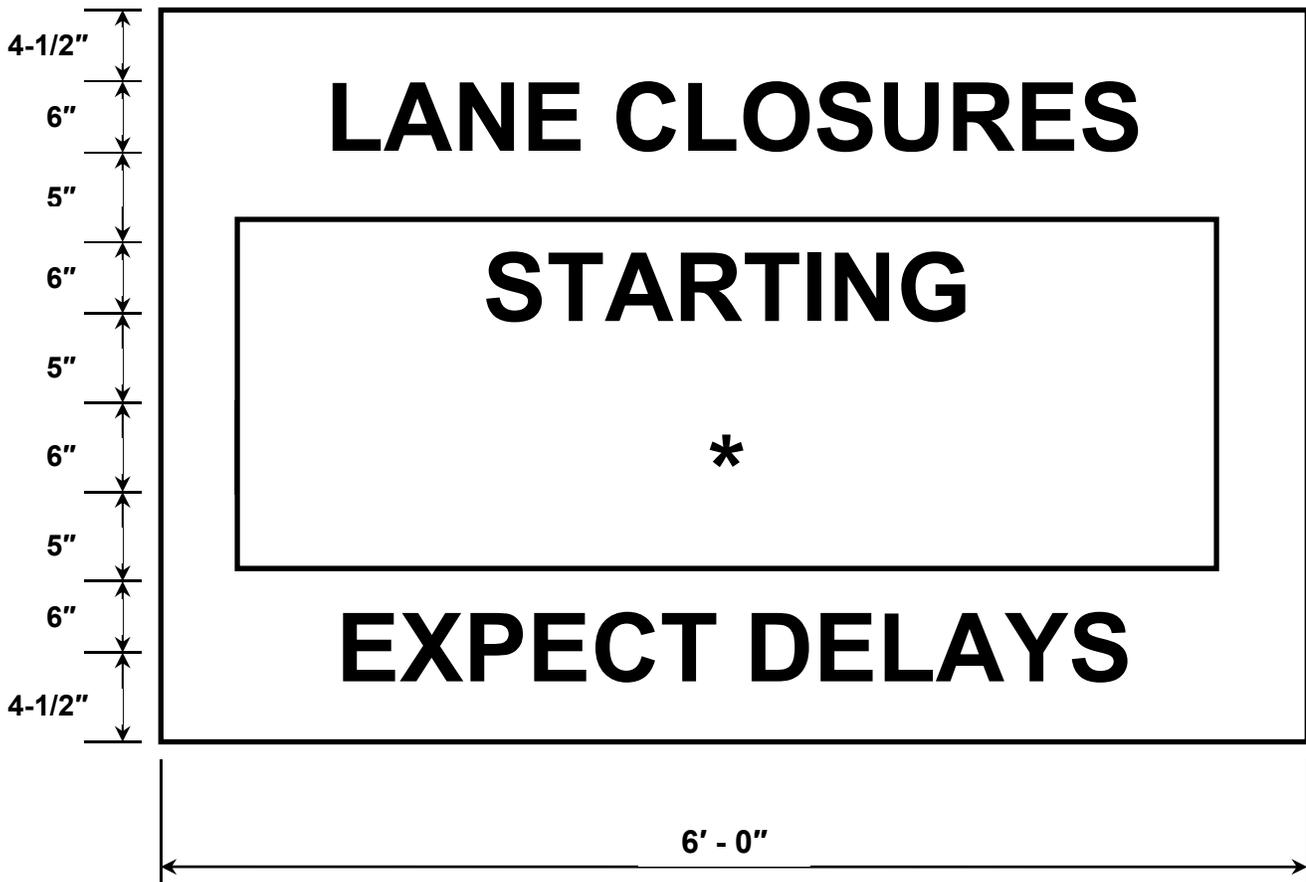
\* Contractor shall provide overlay panel with the date for Start of lane closure. Signs shall be erected a minimum of one (1) week in advance of the start of the work. Overlay panel shall be removed soon after start of construction.
