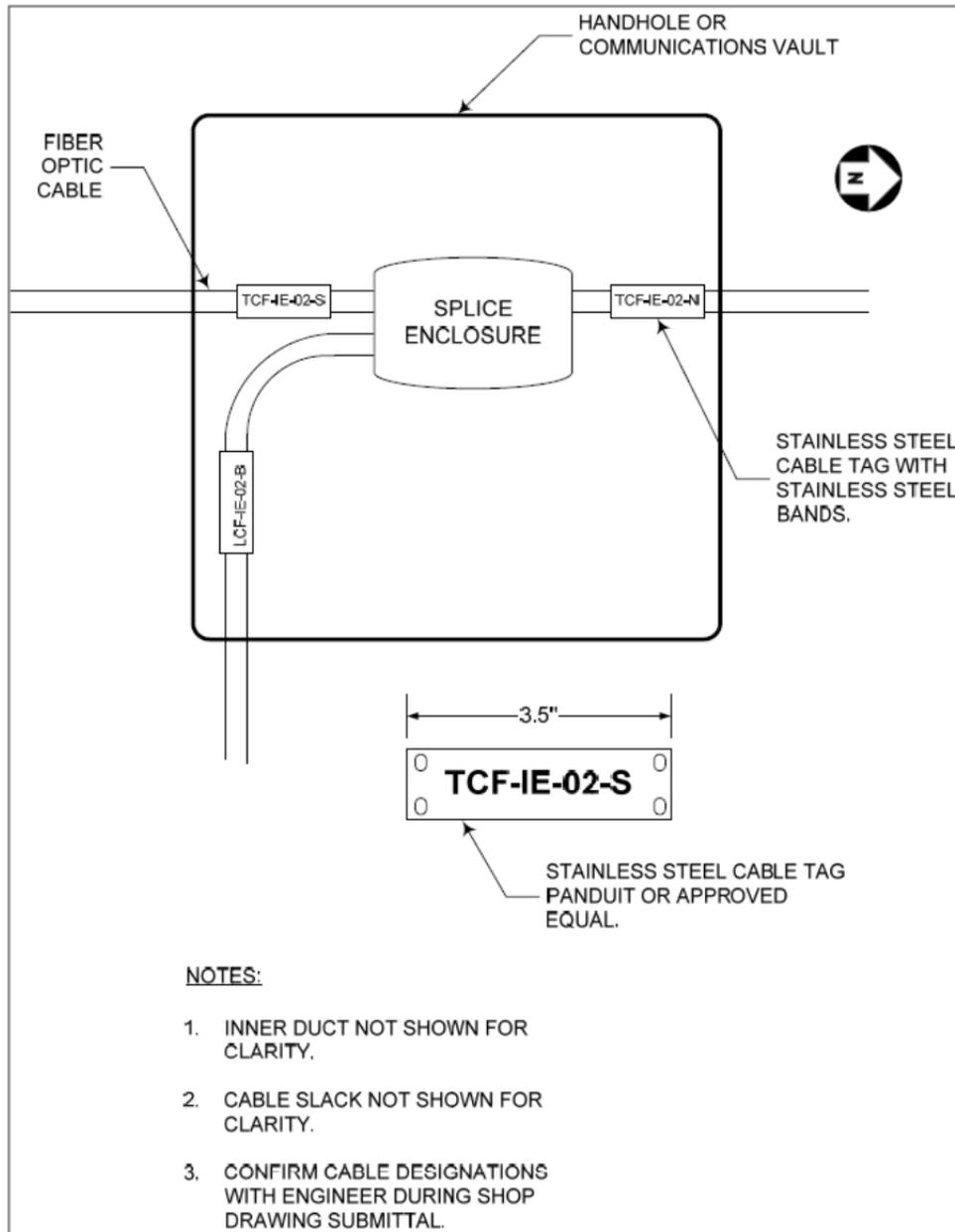
Label the destination of each trunk cable onto the cable in each manhole/handhole, pull/junction box, security building, vault or cable termination panel.
