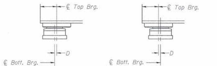
SETTING ANCHOR BOLTS AT EXP. BRG. (Move bott. brg. away from fixed brg.) (Move bott. brg. toward fixed brg.)
