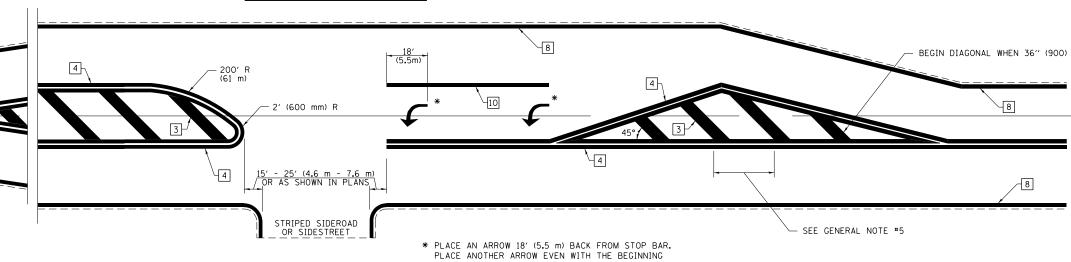
\* PLACE AN ARROW 18' (5.5 m) BACK FROM STOP BAR. PLACE ANOTHER ARROW EVEN WITH THE BEGINNING OF THE SOLID WHITE LINE. SPACE ADDITIONAL ARROWS EVENLY UP TO 80' (24.4 m) MAXIMUM SPACING. USE MINIMUM OF 2 ARROWS.
