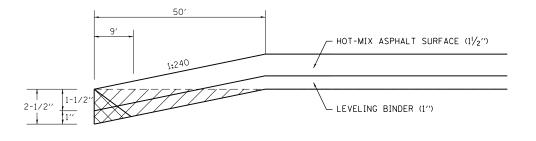
PCC SURFACE REMOVAL BUTT JOINT TEMPORARY RAMP
