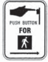
R10-3 THE PEDESTRIAN PUSH-BUTTON SIGNS SHALL BE INCLUDED IN THE COST OF THE ACCESSIBLE PEDESTRIAN SIGNALS. PEDESTRIAN PUSH-BUTTON SIGN DETAIL
