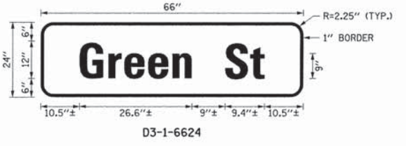
MAST ARM MOUNTED STREET NAME SIGN DETAILS
