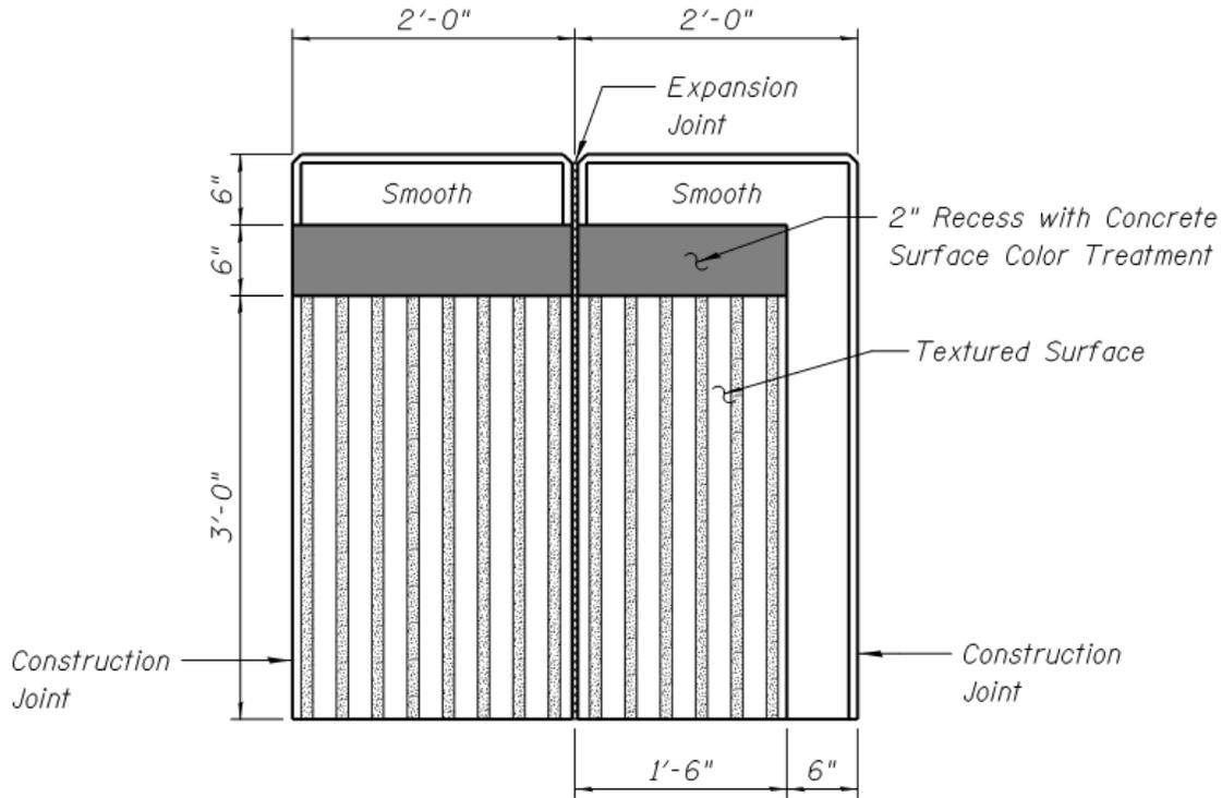
*Include one horizontal and one vertical liner joint within textured surface.*
