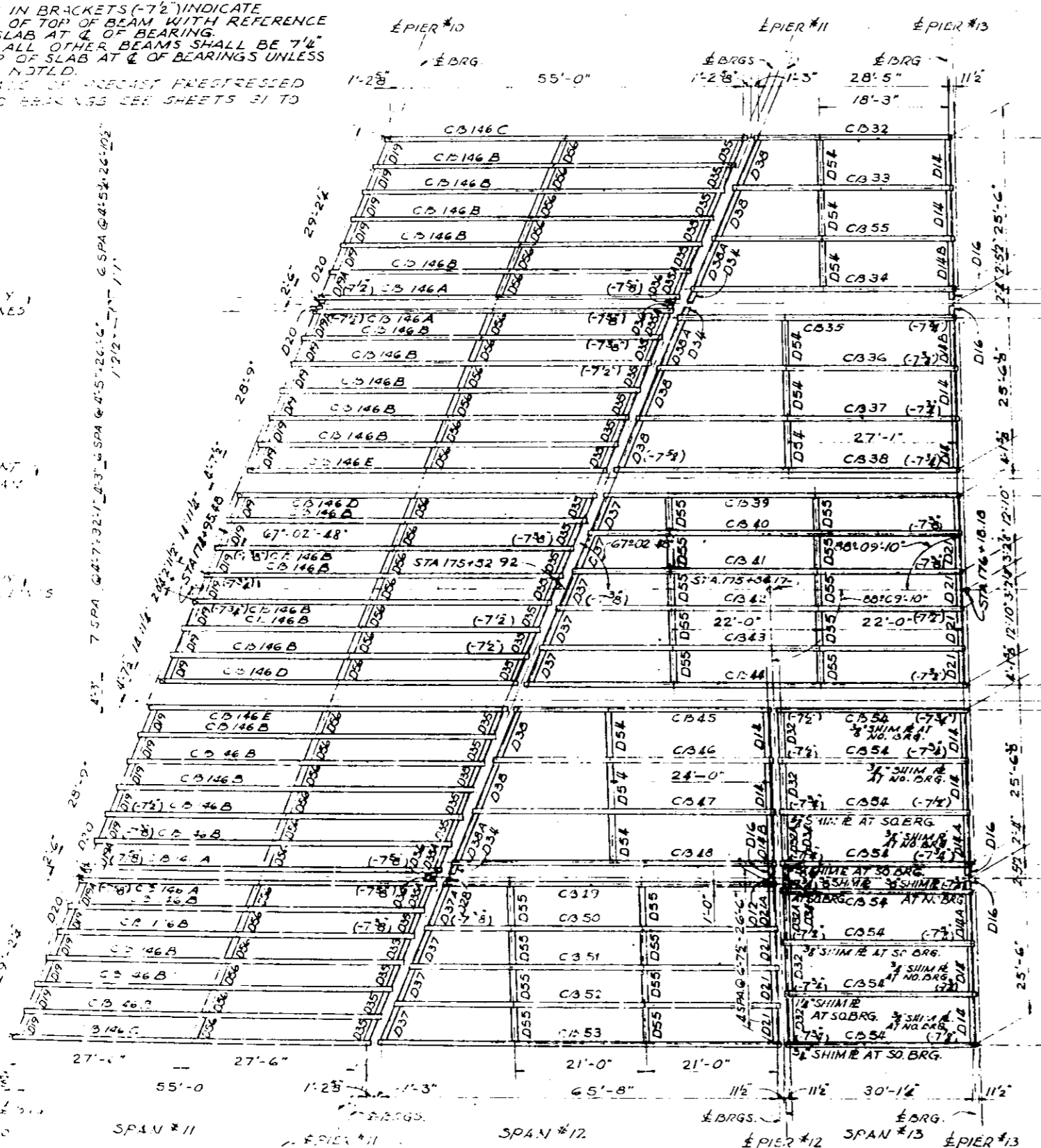
FRAMING PLAN SPANS #11 TO 13 INCL. SCALE: 1/2" = 1'-0"
