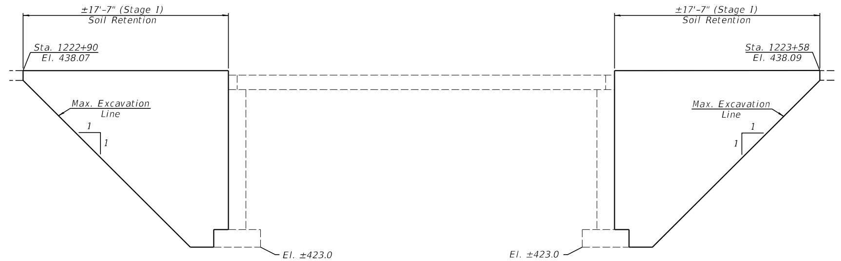
TEMPORARY SOIL RETENTION SYSTEM (Looking Upstream)
