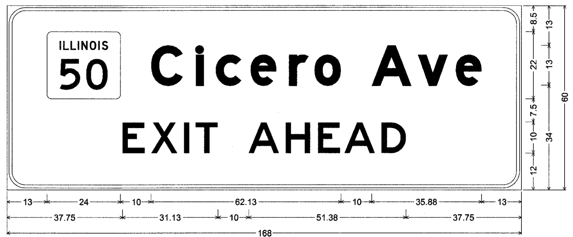
E1-1 (1.4) Ill; 6.00" Radius, 1.00" Border, 0.63" Indent, White on Green; [Cicero] E Mod; [Ave] E Mod; [EXIT] E; [AHEAD] E;
