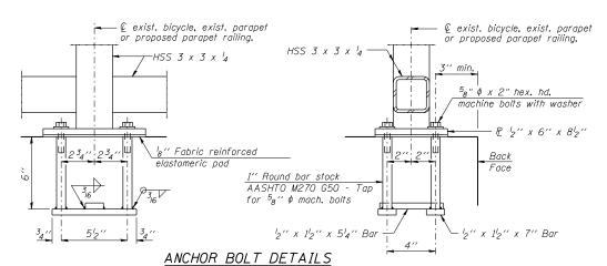
In lieu of the cast-in-place anchor device shown, the Contractor has the option of drilling and setting  $^58''$   $^{\circ}$  anchor rods according to Article 509.06 of the Standard Specifications. Embedment shall be according to the manufacturer's specifications.
